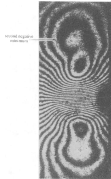
Fig. 6—Enlarged area from the interferogram at time  $21.7\mu\text{s}$  in Fig. 5. The arrow points to the formation of the second negative minimum in the fringe pattern
